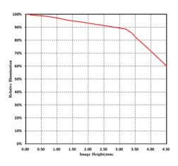
Note: The above curves are the simulate results based on F2.4,  $\beta$ =-0.019, WD=300 mm.
