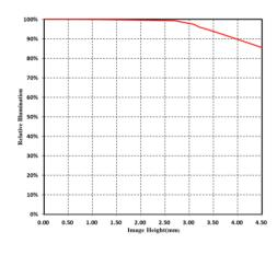
Note: The above curves are the simulate results based on F2.4,  $\beta$ =-0.039, WD=400 mm.
