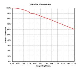
Note: The above curves are the simulate results based on F1.8,  $\beta$ =-0.125, WD=300 mm
