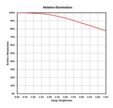
Note: The above curves are the simulate results based on F2.8,  $\beta$ =-0.126, WD=400 mm
