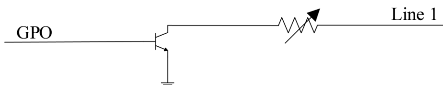
Figure 10-3 Line 1 Internal Circuit
