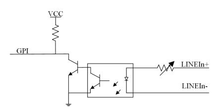
Figure 3-1 Internal Circuit of Input Signal
