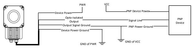
Figure 3-8 Output Signal Connecting to PNP Device
