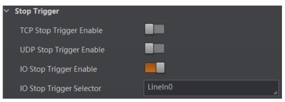
Figure 8-33 IO Stop Trigger
