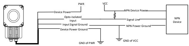
Figure 3-7 Input Signal Connecting to NPN Device with Pull-Up Resistor
