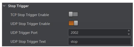
Figure 8-32 UDP Stop Trigger
