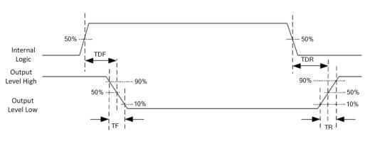
Figure 3-4 Output Logic Level
