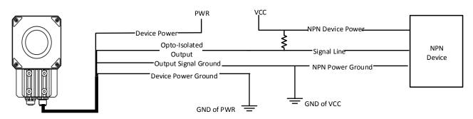
Figure 3-10 Output Signal Connecting to NPN Device with Pull-Up Resistor
