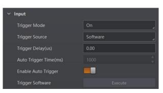
Figure 8-24 Set and Execute Software Trigger Mode
