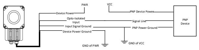
Figure 3-5 Input Signal Connecting to PNP Device
