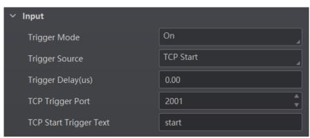
Figure 8-27 Set and Execute TCP Trigger Mode
