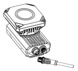
Figure 4-3 Gigabit Ethernet Interface Wiring
