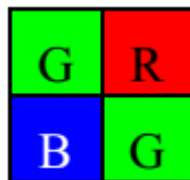
Figure 11-6 Bayer GR Pixel Pattern
