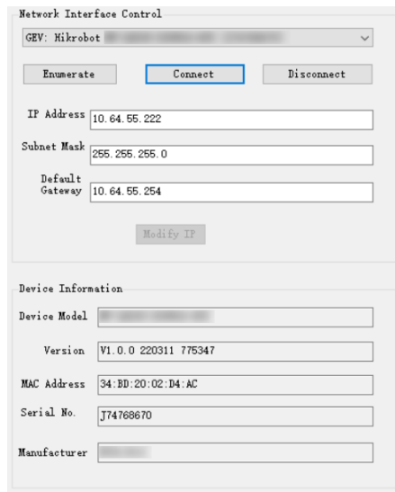
Figure 7-3 Network Interface Connection
