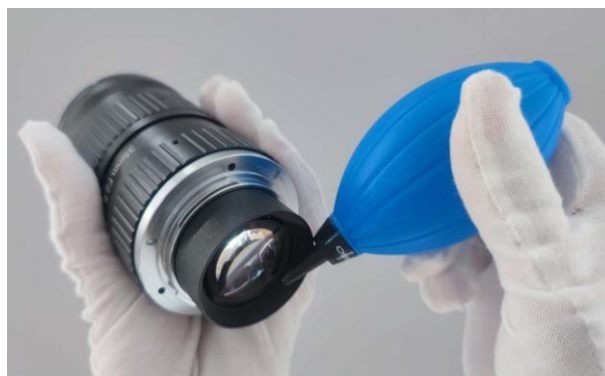
Figure 2-1 Cleaning by Rubber Dust Air Blower
